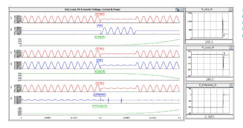
SIMULATION RESULTS FOR POWER-HARDWARE-IN-THE-LOOP TESTING OF A PV MICROINVERTER FOR A 5 CYCLE L-G FAULT
