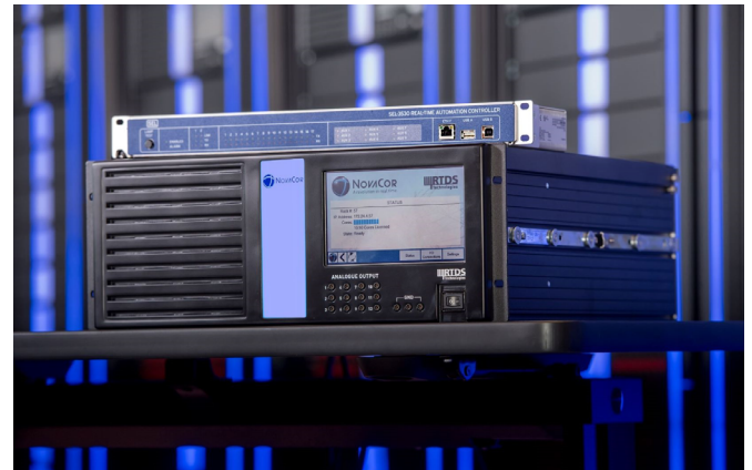
Testing a real-time automation controller for microgrid control with the RTDS Simulator
