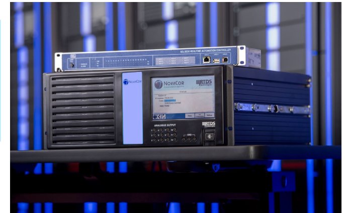
Testing a real-time automation controller for microgrid control with the RTDS Simulator
